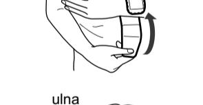
Make sure that the wrist cuff does not cover the protruding part of the wrist bone (ulna) on the outside of the wrist.
